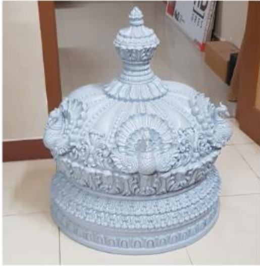
Step 1 - Dome made in FRP
